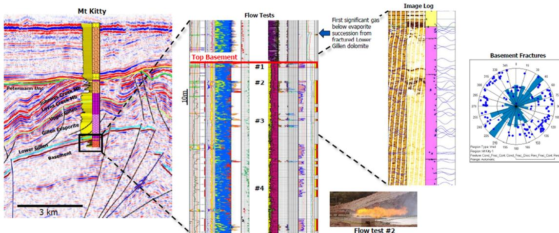
Figure 9. Gas flows from natural fractures in granite and pre-salt carbonates. Mt. Kitty 1 well (Northern Territories, Australia) stratigraphy and flow test results, from [19].
