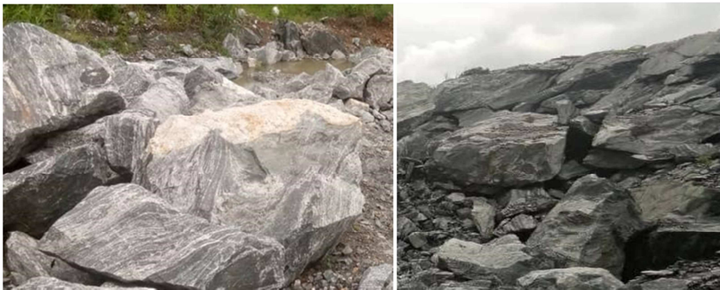
Figure 5. Image showing misfire and back break produced during electrical blasting at Oakyam Quarry.
