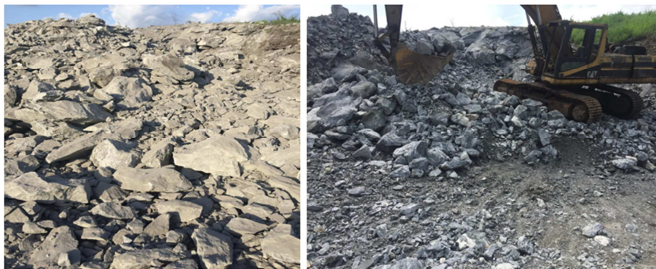
Figure 11. Images of fragmented rocks using an improved blasting technique.
